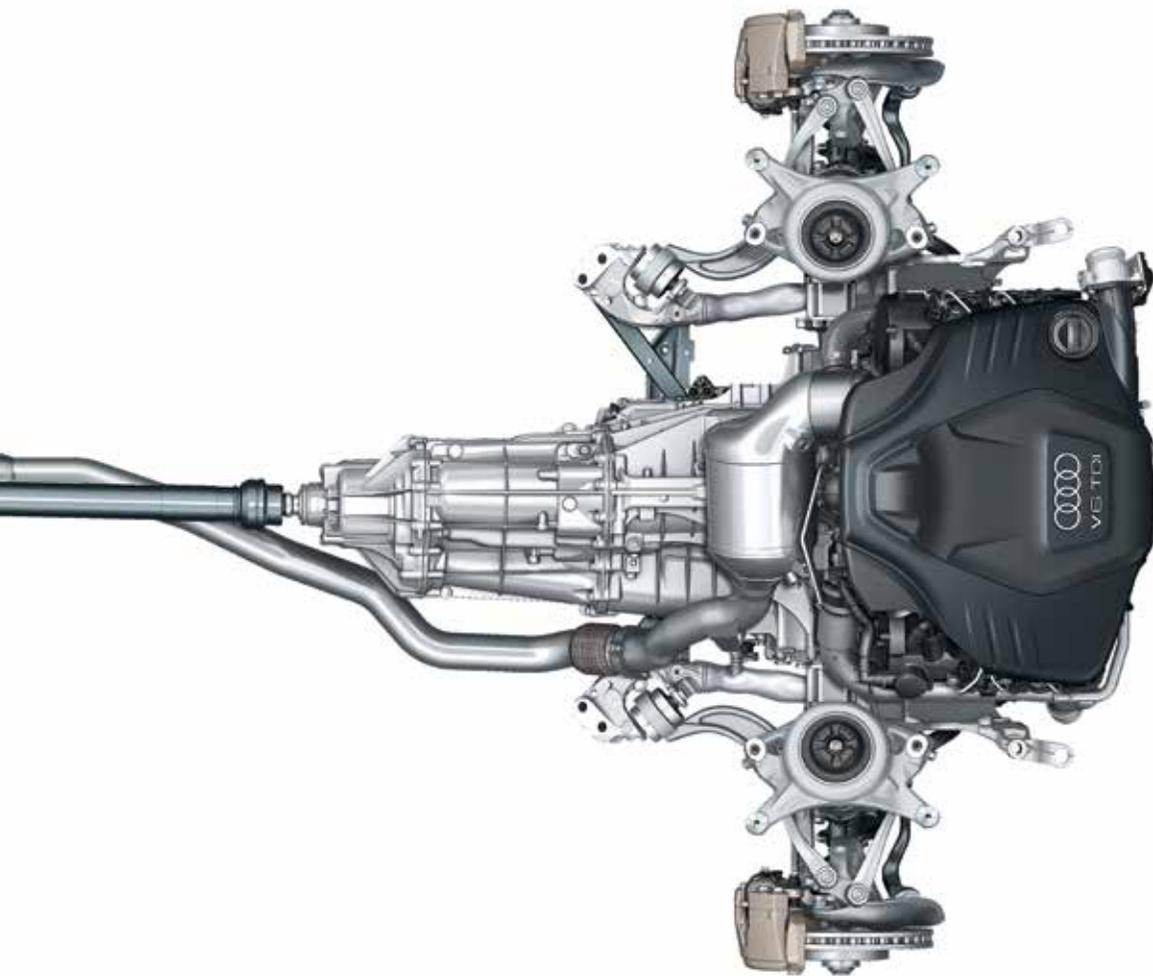
In the Audi A5 Coupé, asymmetric dynamic torque distribution continuously distributes drive power between the front and rear axles, depending on weather conditions, road surface and gradient. This leads to greater flexibility and an enhanced, sportier drive.
